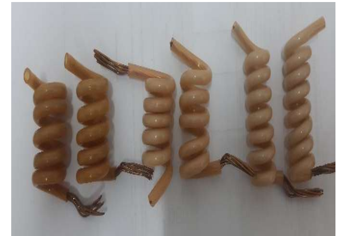
Bending Test After Ageing 150°C, 240 hours
