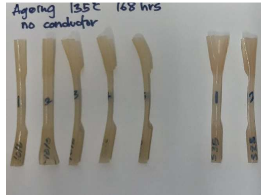
After Ageing 135°C, 168 hours without conductor
