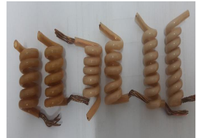
Bending Test After Ageing 150°C, 240 hours
